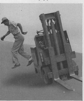
SHADES OF Barney Oldfield, only here we demonstrate with a fork lift. Excessive speed and a fast corner mean an overturned fork lift and probable injury. It has happened here.
